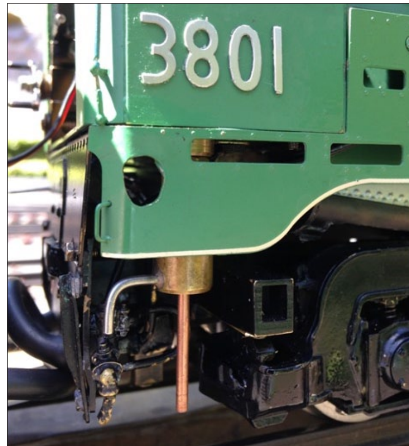
Fig 2 - Water Gauge Blow Down Valve
