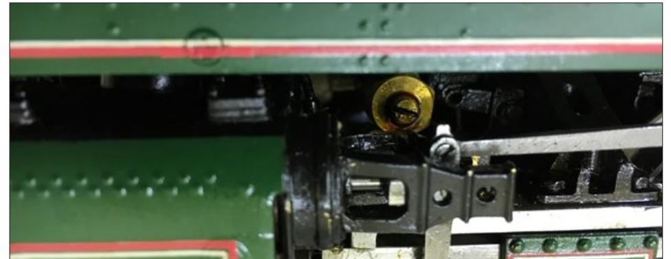
Fig 5 - Lubricator Adjusting Screw (Clockwise = Close)
